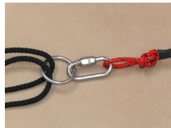
Use the Shackle to attach the Sea Anchor
